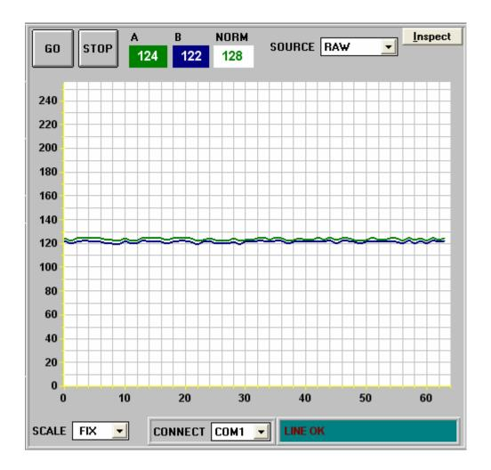
Fields A and B in the above picture show the current measured values of the sensor.
