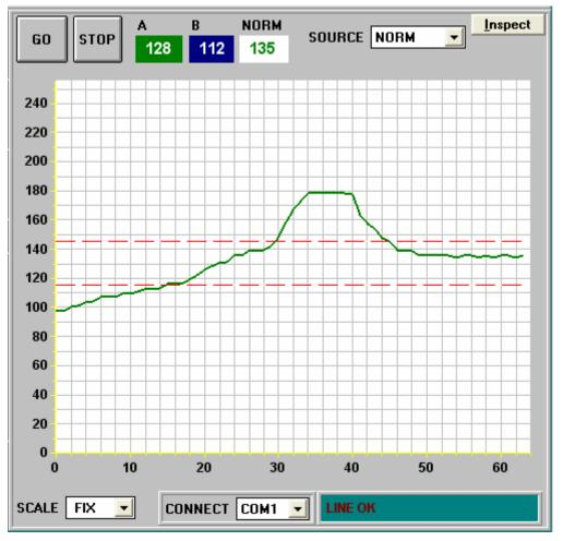
The NORM field shows the value that is standardised by the software, which is formed from the two signals A and B.
